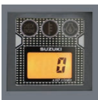
Tachometer with warning indicators
